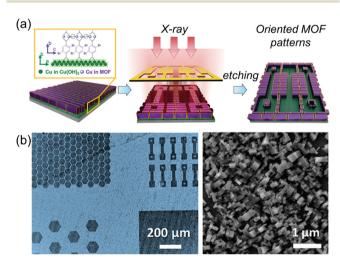
Fig. 4 (a) A schematic illustration of the patterning of oriented MOF films via photolithography. (b) Optical image of micropatterned  $Cu_2[(Br_2BDC)_x(BDC)_{1-x}]_2DABCO$  oriented film on  $Cu(OH)_2$  (left) and SEM image of oriented MOFs in the unexposed area to X-ray (right). Adapted with permission from ref. 75. Copyright 2023, Wiley-VCH.
