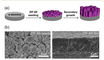
Fig. 2 (a) Schematic illustration of the process for synthesizing an oriented ZIF-69 film on an  $\alpha$ -alumina substrate by seeding ZIF-69 crystals and subsequent secondary growth. (b) SEM image of ZIF-69 seeds on the substrate (left) and cross-section of the oriented ZIF-69 film grown through secondary growth (right). Adapted with permission (part of figures) from ref. 72. Copyright 2011, Elsevier.
