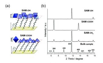
Fig. 5 (a) Schematic illustration of [111] oriented HKUST-1 crystals with -OH SAM and [100] oriented HKUST-1 crystals with the -COOH SAM in the film. (a) XRD patterns of bulk and oriented films of HKUST-1 depending on the SAM functional groups. Adapted with permission from ref. 78. Copyright 2007, American Chemical Society.
