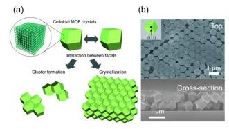
Fig. 19 (a) Scheme of the interaction between ZIF-8 crystal facets driven by capillary forces and van der Waals interactions. (b) SEM images of top view (top) and cross-sectional view (down) of assembled ZIF-8 particles in (111) direction parallel to the out-of-plane direction of Si substrates. Adapted with permission from ref. 107. Copyright 2012, Wiley-VCH.
