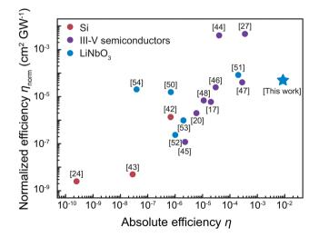
Fig. 4 Comparison of SHG efficiency in Si, III-V semiconductors, and LiNbO<sub>3</sub> metasurfaces.
