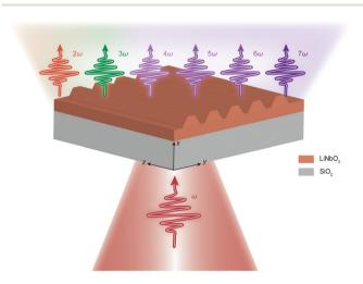
Fig. 1 Schematic of HHG from a LiNbO<sub>3</sub> metasurface supporting guided-mode resonance. When the TE-polarized pump laser is normally incident from the substrate side, the nonlinear harmonic signals from the 2<sup>nd</sup> to 7<sup>th</sup> order are emitted in the transmission direction. The metasurface is composed of a LiNbO<sub>3</sub> grating whose optical axis is along the z-direction situated on a SiO<sub>2</sub>/quartz substrate.
