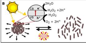
Fig. 1 Schematic illustration showing (A) the "one-pot" preparation of Sb<sub>2</sub>S<sub>3</sub> microrobots using a microwave reactor and (B) their phoretic properties under light irradiation that induce swarming-like behavior. CB and VB stand for conduction and valence bands, respectively.
