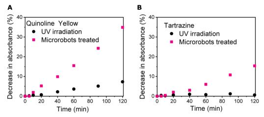
Fig. 5 Photodegradation of food dyes determined by the change in absorbance. Graphs show degradation of quinoline yellow (A) and tartrazine (B) using photocatalytically active microrobots and UV irradiation alongside the control experiment where no microrobots were applied.
