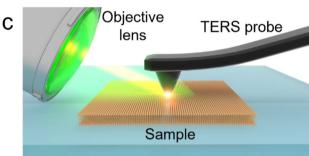
Fig. 1 Schematic illustration of different TERS setups. (a) Bottom illumination, (b) top illumination and (c) side illumination.
