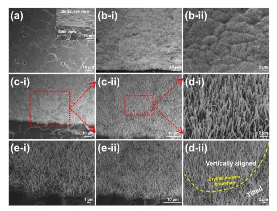
Fig. 5 Scanning electron micrographs: (a) top view of the bare BeO substrate, with an inset showing a bird's-eye view, (b-i and b-ii) low- to highmagnification images of GaN core NWs, (c-i and c-ii) low- to high-magnification images of InGaN/GaN MQW NWs, (d-i and d-ii) images with an emphasis on the vertical development of the NWs, and (e-i and e-ii) images of InGaN/GaN MQW NWs with a focus on the skewed growth. Reproduced with permission from ref. 81. Copyright 2020 ACS publisher.
