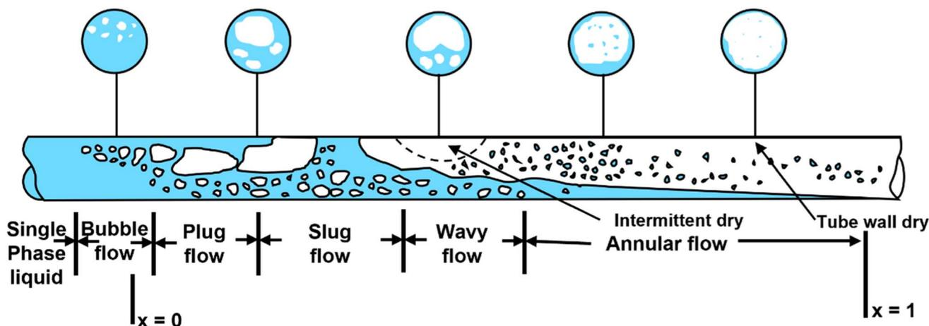
Fig. 7 Subcooled-inlet flow boiling patterns as a function of vapor quality ( $x$ ) showing bubbly, plug, slug, wavy and annular flow followed by dry-out.<sup>120</sup>
