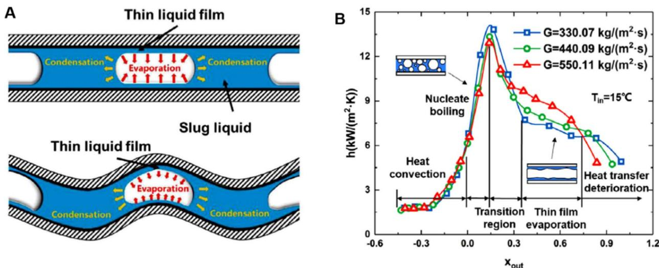
Fig. 9 (A) Top views of confined bubbles in wavy and straight microchannels.<sup>179</sup> (B) Variation of flow boiling HTC ( $h$ ) as a function of outlet vapor quality ( $x_{\text{out}}$ ) for different mass fluxes ( $G$ ) at an inlet saturation temperature ( $T_{\text{in}}$ ) of 15 °C.<sup>179</sup> Reproduced with permission from ref. 179. Copyright 2021 Elsevier.
