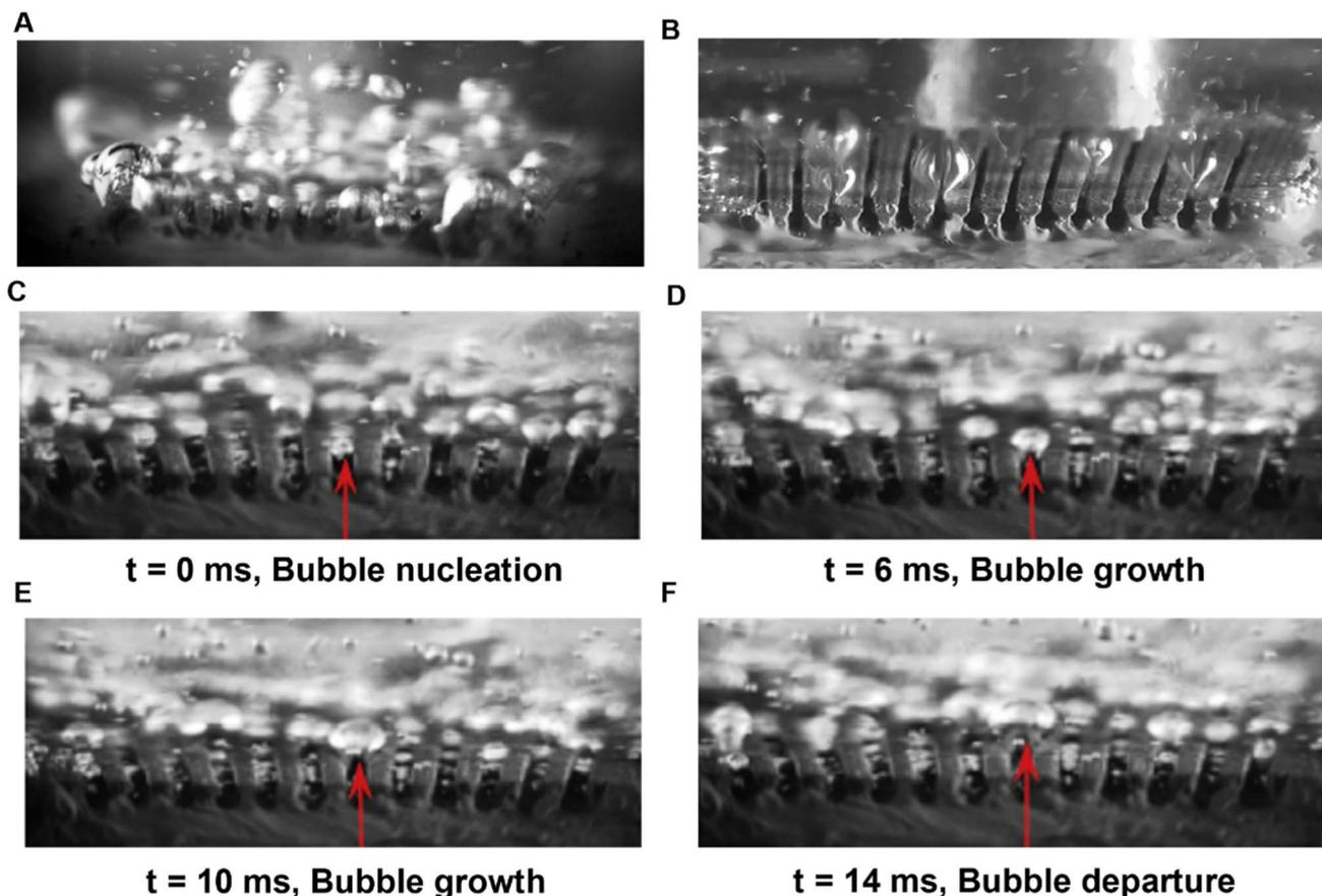
Fig. 4 Optical photograph demonstrating more nucleation for (A) porous structured reentrant cavity surface<sup>88</sup> when compared against (B) non-porous reentrant cavity surface with water as the working fluid.<sup>88</sup> (C–F) Bubble nucleation, growth and departure captured for porous reentrant cavity surface with ethanol as the working fluid.<sup>88</sup> Reproduced with permission from ref. 88. Copyright 2016 Elsevier.
