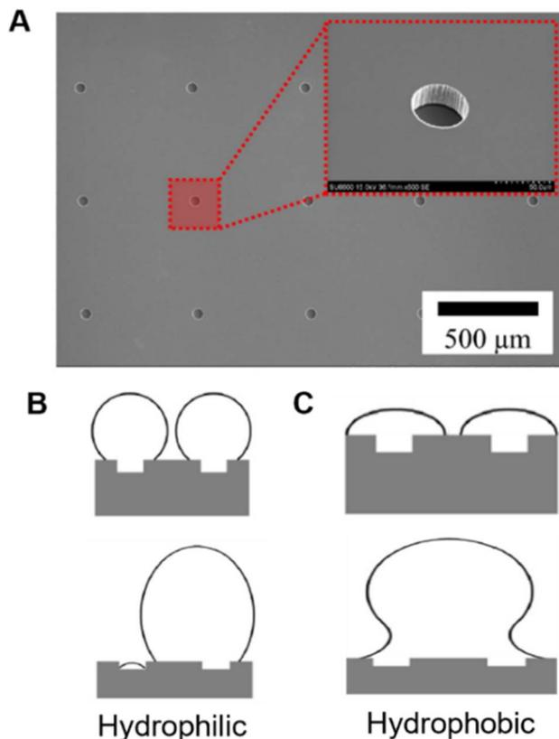
Fig. 3 (A) SEM images of micro-hole patterned surface.<sup>67</sup> Bubble nucleation and growth on microhole patterned (B) hydrophilic<sup>67</sup> and (C) hydrophobic surfaces at low wall superheats.<sup>67</sup> Reproduced with permission from ref. 67. Copyright 2020 Elsevier.
