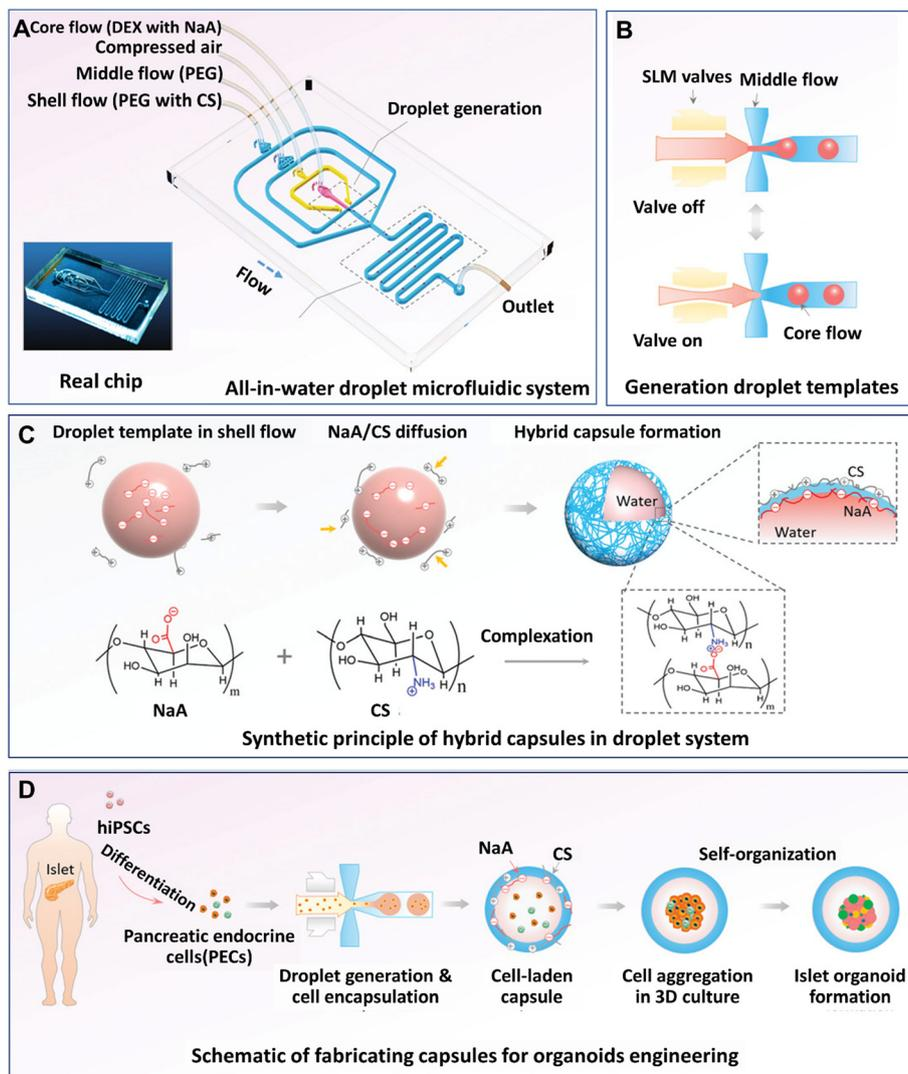
**Fig. 10** Formation and applications of organoids in core-shell microcapsules in a DMF platform. (A) An all-in-water droplet microfluidic system used for organoid generation. (B) Generation of droplet templates controlled by an SLM valve. (C) Core-shell microcapsules generated from a hybrid polymer from alginate and chitosan. (D) Schematic of the fabrication of capsules for organoid engineering. Reproduced from ref. 84 with permission from John Wiley & Sons Inc., copyright 2020.
