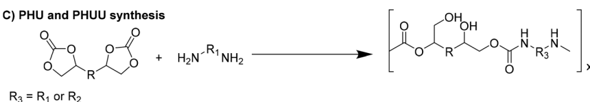
Fig. 11 Polyhydroxiuethane (PHU) and PHUU synthetic route.
