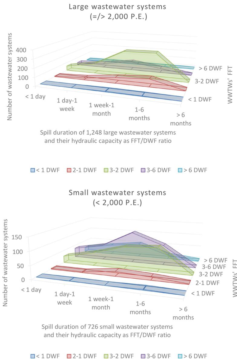
**Fig. 3** Spill duration of wastewater systems during 2021 and the flow to full treatment (FFT) of their wastewater treatment works (WWTWs) expressed as multiples of dry weather flow (DWF) in five categories: spilled up to a day ( $\leq 1$  d); spilled between a day and a week (1 d–1 w); spilled between a week and 1 month (1 w–1 m); spilled between 1 and 6 months (1 m–6 m); and spilled more than 6 months ( $> 6$  m).
