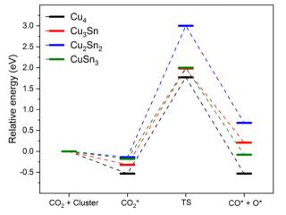
Fig. 4 Reaction pathway for  $CO_2$  dissociation into  $CO^*$  and  $O^*$  over  $Cu_4$ ,  $Cu_3Sn$ ,  $Cu_2Sn_2$ , and  $CuSn_3$  clusters. The structures are those of the chemisorbed  $CO_2$ , transition state, and  $(CO^* + O^*)$  on  $Cu_4$ . Blue, brown, and red balls represent metal Cu, C and O atoms, respectively.
