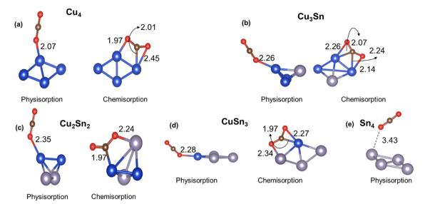
Fig. 3 Lowest energy structures of CO<sub>2</sub> physisorbed and chemisorbed on monometallic and bimetallic Cu-Sn clusters. Blue, grey, brown, and red balls represent Cu, Sn, C and O atoms, respectively
