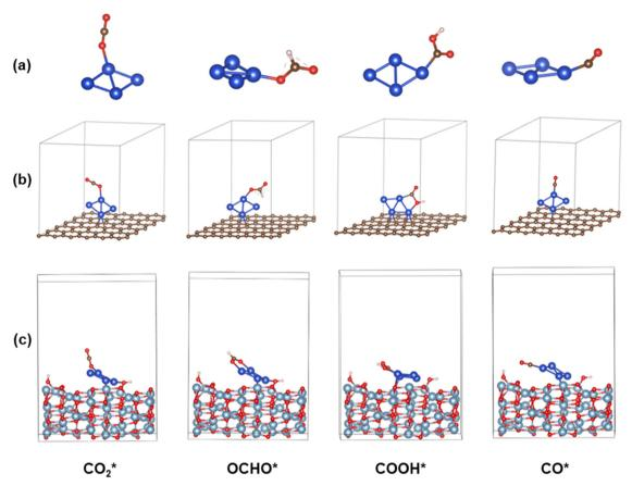
Fig. 7 Optimized structures of the  $CO_2^*$ , OCHO\*, COOH\*, and CO\* intermediates on (a)  $Cu_4$ , (b)  $Cu_4$ /graphene, and (c)  $Cu_4/\gamma$ -Al<sub>2</sub> $O_3$  (110). Blue, grey, brown, red and white balls represent Cu, Al, C, O and H atoms, respectively.
