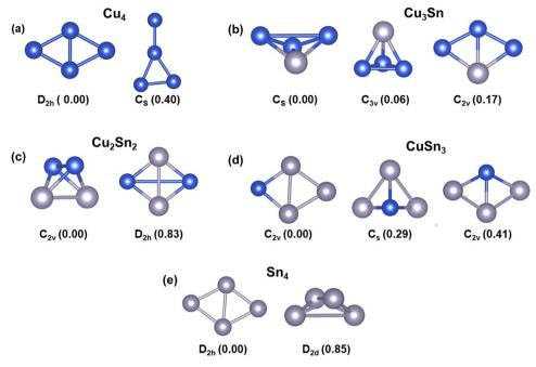
Fig. 1 The lowest energy isomers of the four-atom  $Cu_{4-n}Sn_n$  (n = 0-4) clusters: (a)  $Cu_4$ ; (b)  $Cu_3Sn_3$ ; (c)  $Cu_2Sn_2$ ; (d)  $CuSn_3$ ; (e)  $Sn_4$ . The symmetry of the structures is given at the bottom of each isomer. The values within the parenthesis are the relative energies (in eV) of the cluster relative to the most stable isomer. Blue and grey balls represent Cu and Sn atoms, respectively.
