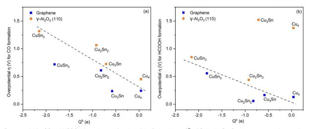
Fig. 8 Overpotential for CO and HCOOH formation as a function of the Bader charge, Q<sup>b</sup>, of Cu in the Cu–Sn clusters supported on graphene (blue) and  $\gamma$ -Al<sub>2</sub>O<sub>3</sub> (orange). The dashed black lines in both figures serve as a guide to the eye.
