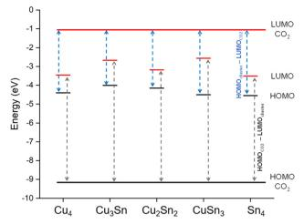
Fig. 2 The HOMO (black line) and LUMO (red line) energy levels of monometallic and bimetallic tetrahedral Cu–Sn clusters compared to that of  $CO_2$ . The dark grey dashed line represents the energy difference between the HOMO of  $CO_2$  and the LUMO of the clusters. The blue dashed line is the energy difference between the HOMO of the clusters and the LUMO of  $CO_2$ .
