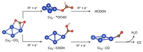
Fig. 5 Reaction pathways for the two proton/two electron (2H<sup>+</sup>/2e<sup>-</sup>) CO<sub>2</sub> reduction reaction to carbon monoxide (CO) and formic acid (HCOOH) showing the optimised structures of the intermediates on Cu<sub>4</sub>. Blue, brown, red and white balls represent metal Cu, C, O and H atoms, respectively.
