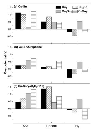
Fig. 10 Overpotential for the electrocatalytic formation of CO, HCOOH and  $H_2$  on (b) isolated  $Cu_nSn_{2-n}$ , (b)  $Cu_nSn_{2-n}$ /graphene, and (c)  $\gamma$ -Al<sub>2</sub>O<sub>3</sub>.
