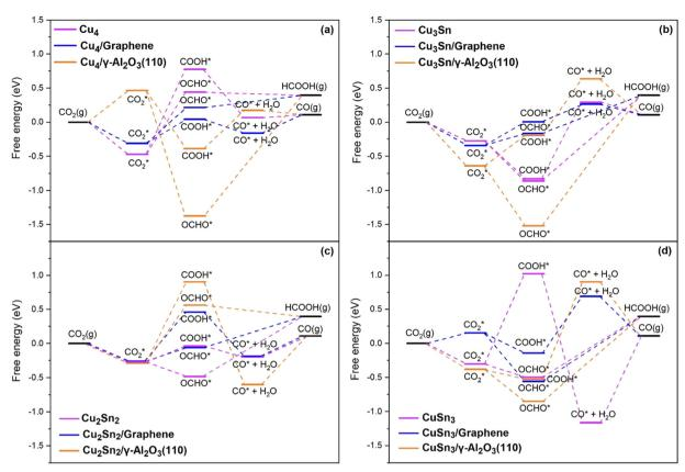
Fig. 6 Gibbs free energy diagram for the eCO<sub>2</sub>R pathways to HCOO and CO on the (a) Cu<sub>4</sub>, (b) Cu<sub>3</sub>Sn, (c) Cu<sub>2</sub>Sn<sub>2</sub>, and (d) CuSn<sub>3</sub> clusters. Reduction pathways on isolated  $Cu_{4-n}Sn_n$  (n=1-3) clusters (light purple) and clusters supported on graphene (blue) and on the partially hydroxylated (110) surface of  $\gamma$ -Al<sub>2</sub>O<sub>3</sub> (orange).
