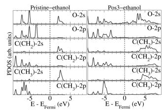
Fig. 5 PDOSs for the 2 s and 2 p orbitals of oxygen and the carbon atoms of  $CH_2$  and  $CH_3$  ethanol radicals before (left) and after (right) ethanol adsorption onto  $Pt_{38}$  on the Pos3 configuration. The data correspond to the optimized configurations and the Fermi level is at zero energy, as indicated by the vertical dashed line.
