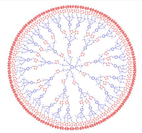
Fig. 7 Planar representation of an 81-ferrocene dendrimer, with equivalent terminal groups, that can serve as battery catholyte.
