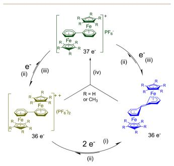
Scheme 8 Electron transfer (ET) processes of diphenyl diiron complexes of biphenyl in THF• (i) LiAlH<sub>4</sub>,  $-80~^{\circ}$ C; (ii) O<sub>2</sub>, NaPF<sub>6</sub>; (iii) Na/Hg, 20  $^{\circ}$ C; (iv) comproportionation, 20  $^{\circ}$ C. $^{70}$  as shown by the X-ray crystal structure of the blue complex  $(R = CH_3)$ .
