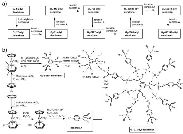
Scheme 6 CpFe $^+$ -induced arene activation for the synthesis of the  $G_0$ -9-allyl dendritic core and dendron A towards the multiple-generation divergent construction of large poly-allyl-terminated dendrimers following  $1 \rightarrow 3$  branching until the 9th generation.
