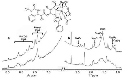
Fig. 20  $^{1}$ H NMR spectroscopic (600 MHz) analysis (a) > 6 ppm and (b) < 3 ppm of AuNP-encapsulated docetaxel (9.5 molecules per Au atom) in H<sub>2</sub>O. Upper traces: docetaxel only; lower traces: docetaxel-AuNPs. Signal assignments were carried out by comparison with the spectrum in DMSO. Note that the solubility of docetaxel alone in H<sub>2</sub>O is by far too low to record a spectrum in this solvent without AuNPs. Reproduced with permission from ref. 143. Copyright 2011 Wiley-VCH.
