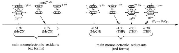
Redox potential scale of useful late transition-metal sandwich complexes as redox reagents.
