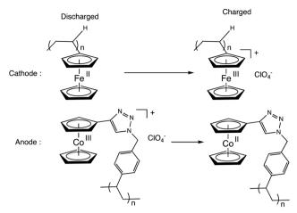
Scheme 10 Electrode reactions in a recent RFBs based on ferrocene polymer as catholyte and cobaltocenium salt as anolyte (driving force: 1.3 V). Electrons are transported by ClO<sub>4</sub><sup>-</sup> anions.
