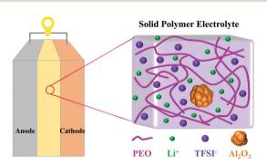
Structures of the solid-state battery and SPE filled with Al<sub>2</sub>O<sub>3</sub>.
