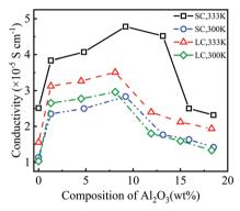
Fig. 4 Conductivities of SPE with different mass fractions of Al<sub>2</sub>O<sub>3</sub>.
