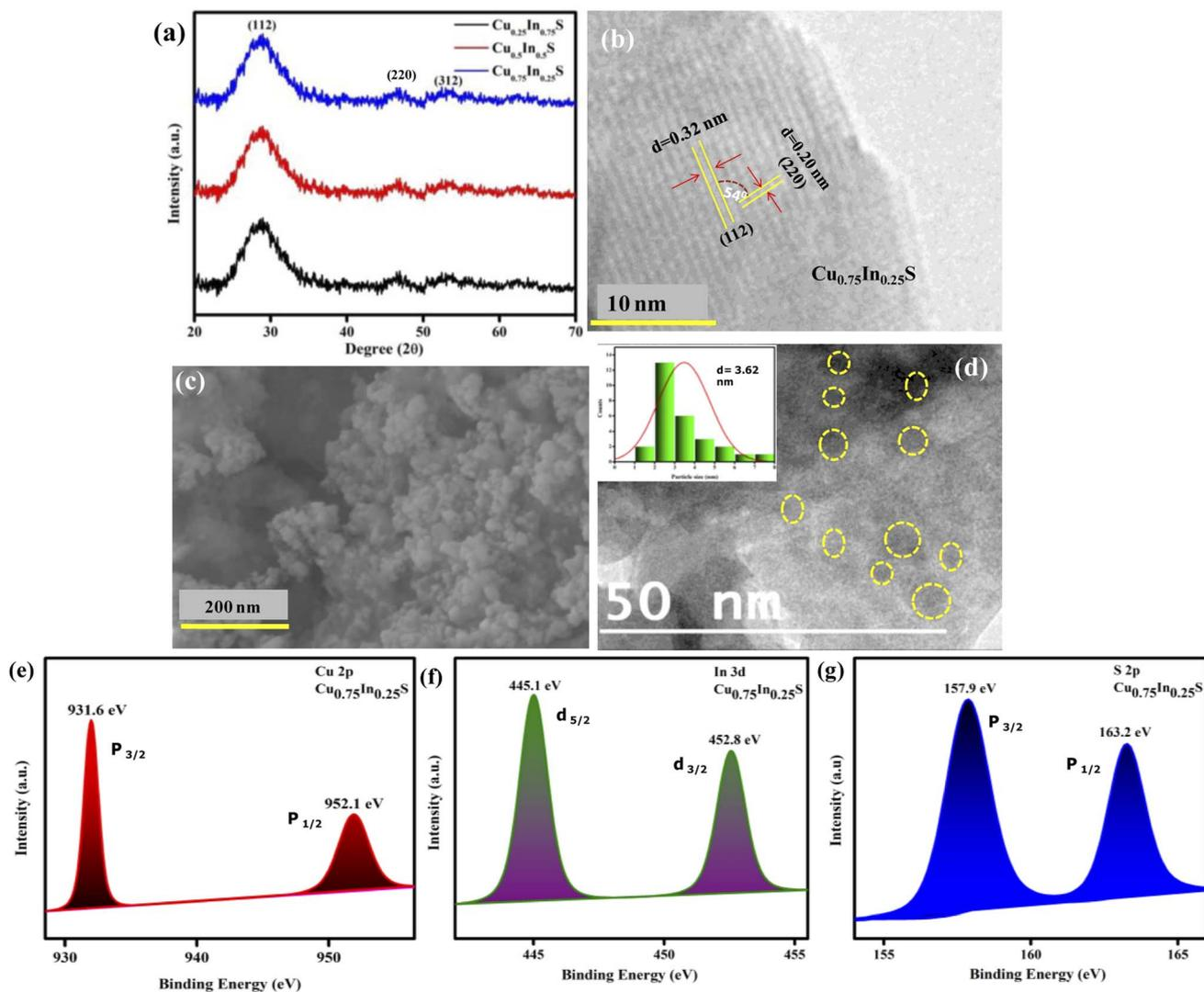
Fig. 1 Structural and compositional characterization: (a) XRD pattern of  $\text{Cu}_x\text{In}_{1-x}\text{S}$  QDs with 3 different molar ratios 0.75 : 0.25, 0.50 : 0.50, and 0.25 : 0.75 of Cu : In, respectively (b) fringe pattern, (c) FESEM and (d) HRTEM images of  $\text{Cu}_{0.75}\text{In}_{0.25}\text{S}$  QD; (e) XPS analysis spectra of Cu 2p, (f) In 3d, and (g) S 2p elements in  $\text{Cu}_{0.75}\text{In}_{0.25}\text{S}$  QD.
