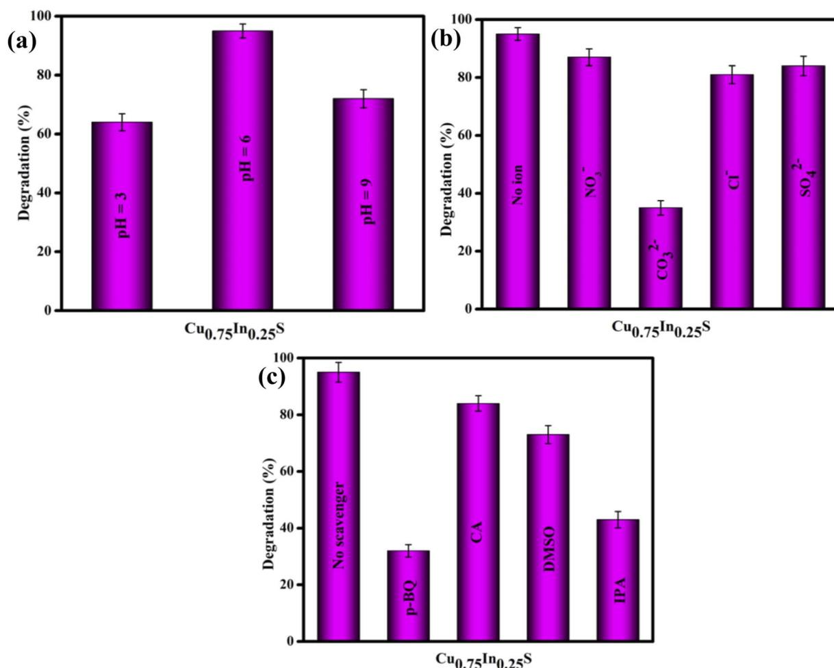
Fig. 5 Degradation efficiency of GMF over 10 ppm  $\text{Cu}_{0.75}\text{In}_{0.25}\text{S}$  photocatalyst on different (a) pH solutions, (b) anions, and (c) scavengers.
