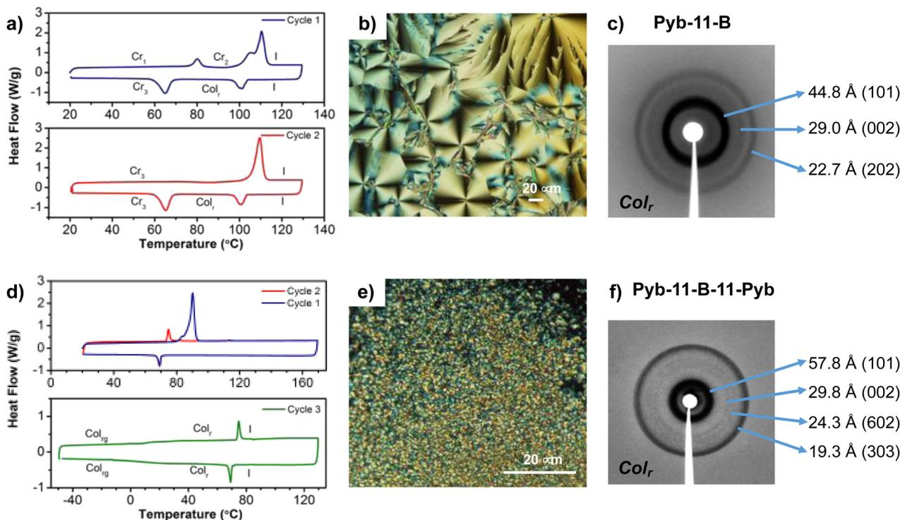
Fig. 2 DSC thermograms and first and second heating/cooling cycles of Pyb-11-B (a) and Pyb-11-B-11-Pyb (d); POM textures of Pyb-11-B at 104 °C ( $Col_r$  phase) (b) and Pyb-11-B-11-Pyb at 74 °C ( $Col_r$  phase) (e); and XRD patterns of the mesophases of Pyb-11-B,  $Col_r$  phase at 102 °C, (c) and Pyb-11-B-11-Pyb,  $Col_r$  phase at room temperature (f).
