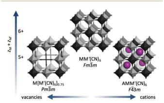
Fig. 1 The crystal structure of Prussian blue analogues. If the charges of the transition metals  $(z_{\rm M}+z_{\rm M'})$  sum to 6, the ordered MM'(CN) $_{\rm 6}$  is formed. For lower charges, vacancies or A-site cations are included to give the formulae  $M[M'(CN)_6]_{y<1}$  and  $A_{x>0}M[M'(CN)_6]$ , respectively. M is shown in dark grey, M' in light grey and A in purple.
