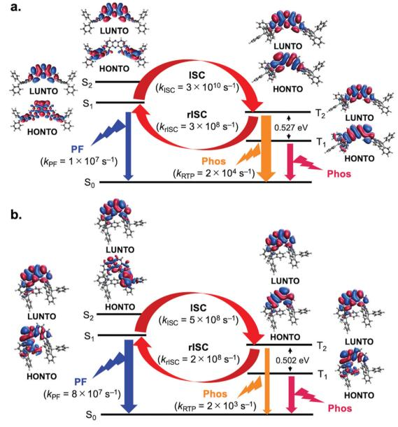
Fig. 6 Schematics showing the NTOs for the first two singlet and triplet states as well as rate estimates for different photophysical processes for compounds (a)  $\bf 1$  and (b)  $\bf 4$ . ISC rates correspond to the sum of rates from  $S_1$  to the first 5 triplet states.
