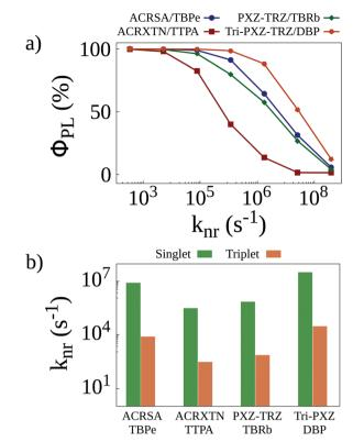
Fig. 3 (a) Photoluminescence quantum yields as a function of the non-radiative decay rate for singlet excitons calculated for simulations with initially only singlet excitons. (b) Non-radiative decay rates that better reproduce experimentally obtained quantum yields<sup>8</sup> as a function of the energy of the emission peak of the four TADF/emitter pairs.
