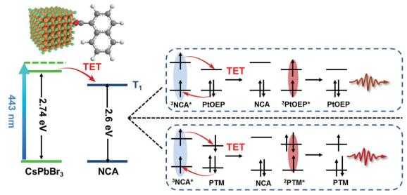
Fig. 1 Sensitization of phosphorescent and radical emitters using NC-transmitter complexes. Photoexcitation of CsPbBr<sub>3</sub> NCs resulted in efficient triplet energy transfer (TET) to the NCA ligands which further translated the energy into PtOEP or PTM-TPA molecules in the bulk solution. Energy transfer from <sup>3</sup>NCA\* to PtOEP or PTM-TPA occurs through electron exchange.
