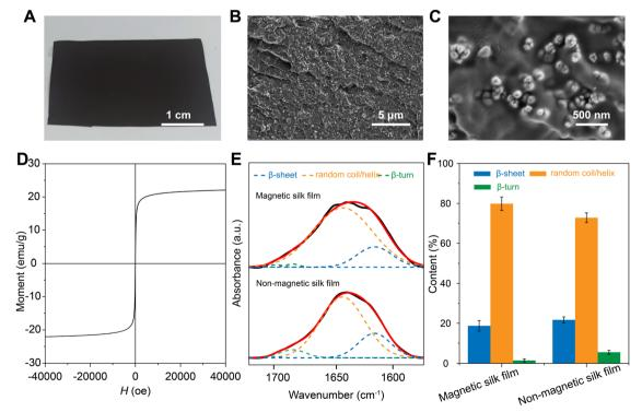
Fig. 3 (A) Photograph of the magnetic silk film. (B and C) SEM images of the magnetic silk film. (D) The magnetization curves of the  $Fe_3O_4$  particles at 37 °C. Inset: Close-up of the hysteresis at H = 0. (E) FTIR spectra of the magnetic and non-magnetic silk films. (F) Secondary structures of the silk proteins in the films from the deconvolution of the amide I region.
