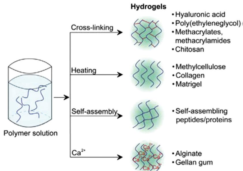
Fig. 11 Different hydrogels and their formation mechanism. Reproduced with permission.<sup>120</sup> Copyright (2018) Elsevier.
