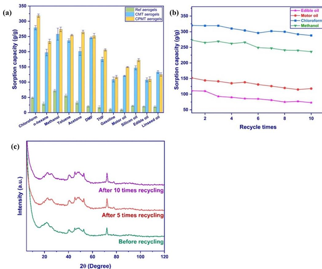
Fig. 10 (a) Sorption capacity of Ref., CMT, and CPMT cryogels for various oils and organic solvents, (b) recyclability of the CPMT cryogel after ten cycles of squeezing, and (c) XRD patterns of CPMT cryogel before and after 5 and 10 times recycling.
