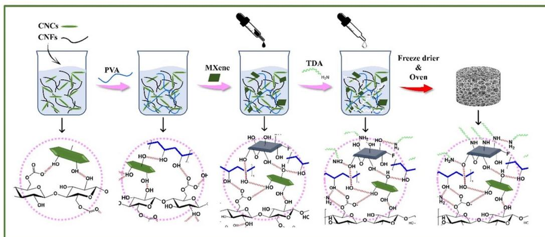
Fig. 5 Preparation of superhydrophobic and cross-linked CPMT cryogel containing MXenes.
