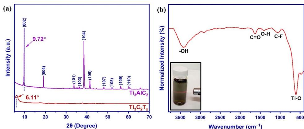
Fig. 1 (a) XRD patterns of  $\text{Ti}_3\text{AlC}_2$  and  $\text{Ti}_3\text{C}_2\text{T}_x$ . (b) FTIR spectrum of  $\text{Ti}_3\text{C}_2\text{T}_x$ . Inset in (b) shows the Tyndall effect of  $\text{Ti}_3\text{C}_2\text{T}_x$  dispersion.
