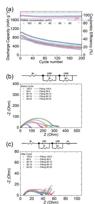
**Fig. 2** Electrochemical analysis of lithium–sulfur cells with the polysulfide cathode and the PMMA-based GPEs with different PMMA: LiTFSI ratios: (a) cyclability for 200 cycles at a cycling rate of C/10; and electrochemical impedance spectra (EIS) (b) before and (c) after cycling.
