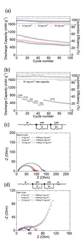
Fig. 3 Electrochemical analysis results of high-sulfur-loading cells: (a) cyclability; (b) rate performance at a sulfur loading of 10 mg cm<sup>-2</sup>; and EIS images (c) before and (d) after cycling
