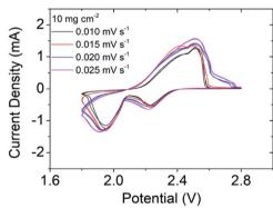
Fig. 4 Cyclic voltammograms of high-sulfur-loading cells: (a) 4 mg  $cm^{-2}$ ; (b) 8 mg cm<sup>-2</sup>; (c) 10 mg cm<sup>-2</sup>.
