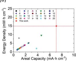
Fig. 5 Comparison of the cell-design parameters and cell-electrochemical performances of lithium-sulfur batteries with the PMMAbased GPE and other GPEs: (a) sulfur loading (mg cm<sup>-2</sup>) and content (wt%) and (b) areal capacity (mA h cm<sup>-2</sup>) and energy density (mW h cm<sup>-2</sup>) based on the whole electrode
