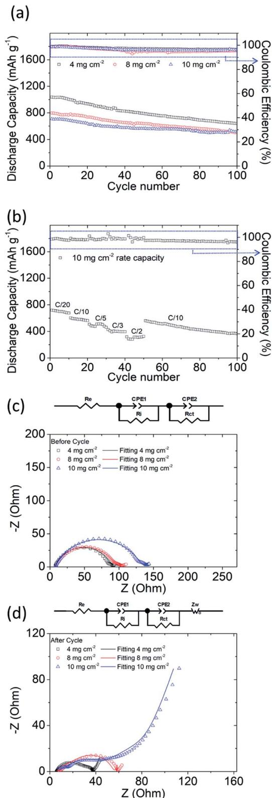
Fig. 3 Electrochemical analysis results of high-sulfur-loading cells: (a) cyclability; (b) rate performance at a sulfur loading of  $10 \text{ mg cm}^{-2}$ ; and EIS images (c) before and (d) after cycling.
