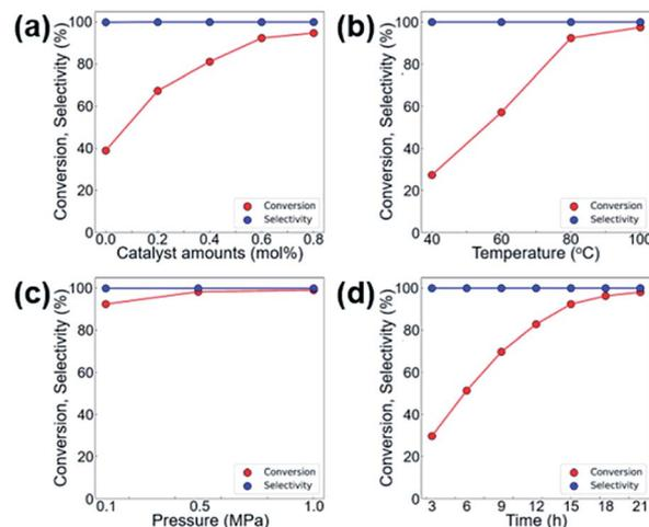
Fig. 6 Effect of various reaction parameters on the cycloaddition of CO<sub>2</sub> and ECH with MOF-801(D) catalysts (a) catalyst amount (co-catalyst 0.5 mol%, 80 °C, 15 h, 0.1 MPa CO<sub>2</sub>), (b) temperature (catalyst 0.6 mol%, co-catalyst 0.5 mol%, 15 h, 0.1 MPa CO<sub>2</sub>), (c) CO<sub>2</sub> pressure (catalyst 0.6 mol%, co-catalyst 0.5 mol%, 80 °C, 15 h), and (d) time (catalyst 0.6 mol%, co-catalyst 0.5 mol%, 80 °C, 0.1 MPa CO<sub>2</sub>).
