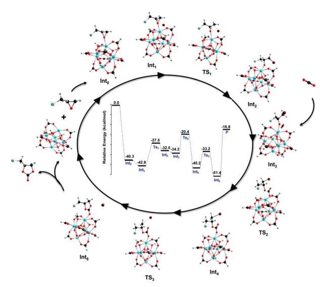
Fig. 8 Relative energy profile for the MOF-801/TBABr catalyzed cycloaddition reaction of CO<sub>2</sub> with ECH to form chloropropene carbonate and the DFT optimized structures of intermediates and transition states.
