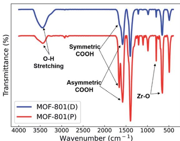
**Fig. 4** FT-IR spectra of MOF-801(D) and MOF-801(P).
