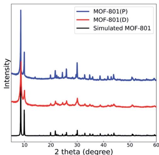
Fig. 2 XRD patterns of MOF-801(D) and MOF-801(P) with simulated MOF-801.
