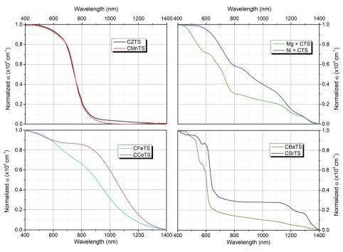
Fig. 3 Normalized absorption spectra for the CXTS films
