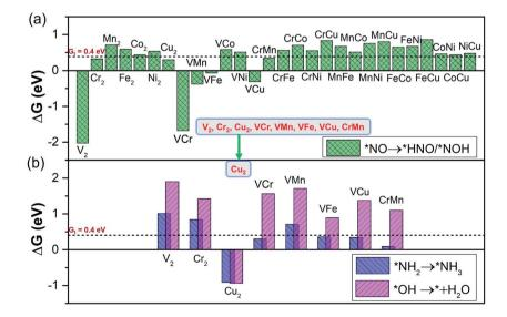
Fig. 4 The screening criterion of "two steps of key hydrogenation process" for NORR activity (step III in Fig. 1b), with the threshold value ( $G_T = \frac{1}{2}$ ) 0.40 eV). (a) The  $\Delta G$  for stabilization of \*NOH/\*HNO species (\*NO  $\rightarrow$  \*NOH/\*HNO) over the 28 DACs. (b) The  $\Delta G$  for destabilization of \*NH<sub>2</sub> and \*OH species (\*NH<sub>2</sub>  $\rightarrow$  \*NH<sub>3</sub> and \*OH  $\rightarrow$  \* + H<sub>2</sub>O) over the 28 DACs.
