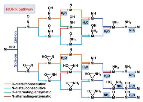
Fig. 3 Schematic depiction of the various pathways for the NORR towards NH<sub>3</sub>. The dotted lines in the adsorbates indicate that bonds may be broken.
