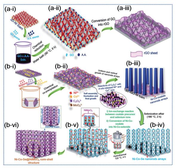
Schematic illustration of the synthesis of the hierarchical hybrid NCSe@NMO@rGO-NF core-shell structure
