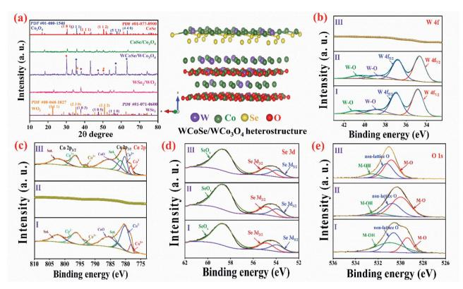
Fig. 3 (a) XRD patterns for the as-synthesized materials and structural alignments of the WCoSe/WCo<sub>3</sub>O<sub>4</sub> heterostructure. XPS spectra of (b) W 4f, (c) Co 2p, (d) Se 3d, and (e) O 1s present in the WCoSe/WCo<sub>3</sub>O<sub>4</sub> heterostructure.
