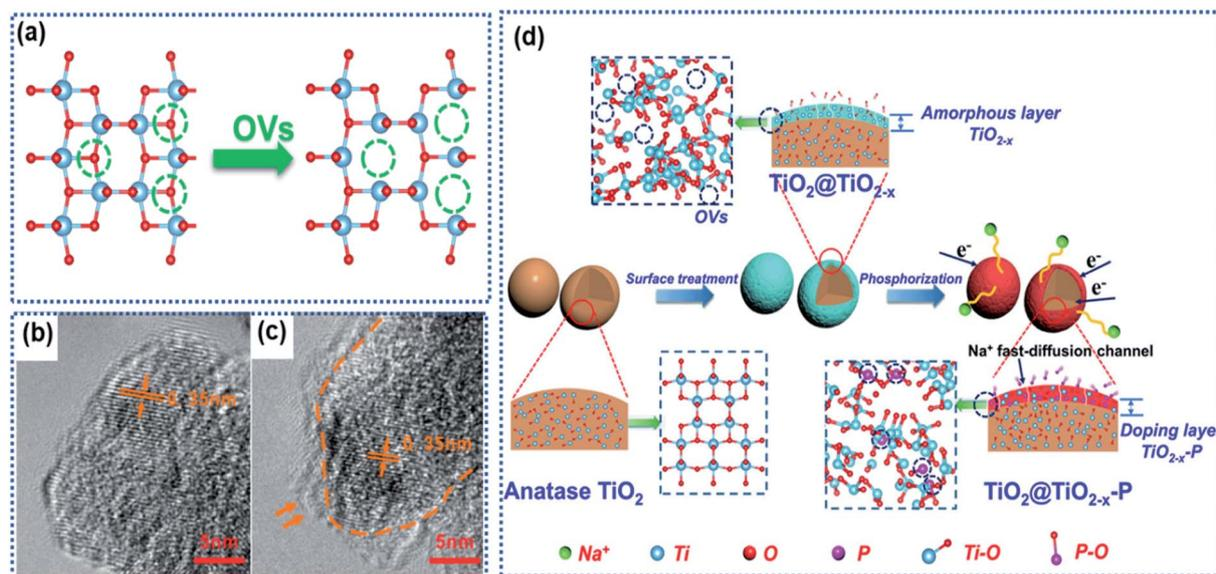
Fig. 2 Surface oxygen vacancies in TiO<sub>2</sub>: (a) schematic illustration of formation of OVVs due to loss of oxygen atoms, (b and c) TEM images of defect-free and defective TiO<sub>2</sub> with surface OVVs,<sup>63</sup> copyright 2016, American Chemical Society. (d) Schematic illustration of surface OV-induced doping of phosphorus (P).<sup>64</sup> Copyright 2019, American Chemical Society.
