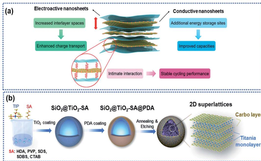
Fig. 7 Microstructure and fabrication of 2D superlattices: (a) schematic illustration of a 2D superlattice facilitating charge transport and storage.<sup>97</sup> Copyright 2020, Royal Society of Chemistry. (b) Schematic illustration of the fabrication of a 2D superlattice consisting of alternative layers of titania and carbon.<sup>35</sup> Copyright 2019, Wiley-VCH.
