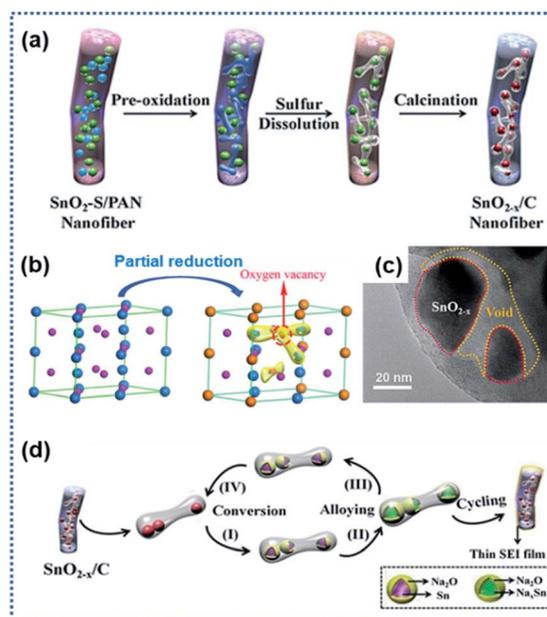
Fig. 3 Surface oxygen vacancies for improving charge transport kinetics of SnO<sub>2</sub>: (a) schematic illustration of the preparation of SnO<sub>2-x</sub>/C nanofibers, (b) illustration of structural transformation from SnO<sub>2</sub> to SnO<sub>2-x</sub>, (c) TEM image of SnO<sub>2-x</sub>/C, and (d) illustration of Na ion intercalation/deintercalation mechanisms in SnO<sub>2-x</sub>/C.<sup>65</sup> Copyright 2018, Wiley-VCH.
