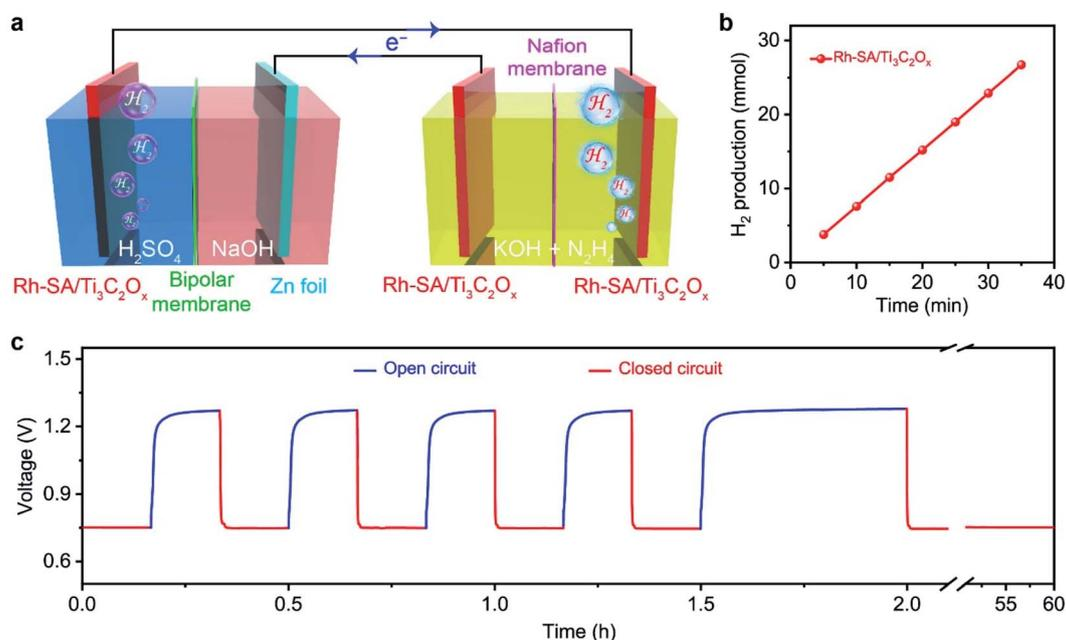
Fig. 6 Self-driven dual hydrogen production system: (a) schematic illustration of the dual hydrogen production system self-driven by the Rh-SA/Ti<sub>3</sub>C<sub>2</sub>O<sub>x</sub> catalyst; (b) the total amount of generated H<sub>2</sub> as a function of the reaction time for this self-driven dual hydrogen production system; (c) the long-time voltage curve of the system at closed/open circuit.
