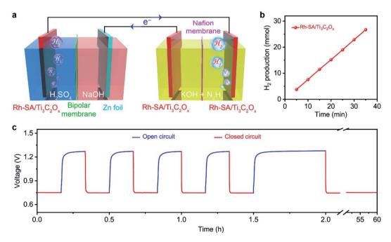
Fig. 6 Self-driven dual hydrogen production system: (a) schematic illustration of the dual hydrogen production system self-driven by the Rh-SA/  $Ti_3C_2O_x$  catalyst; (b) the total amount of generated  $H_2$  as a function of the reaction time for this self-driven dual hydrogen production system; (c) the long-time voltage curve of the system at closed/open circuit.
