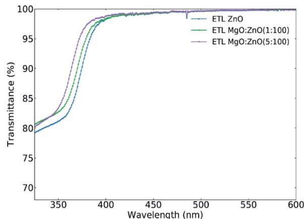
Fig. 3 Transmission spectra of thin films of ZnO and Mg-doped ZnO. There is a blue-shift in the spectrum with increasing Mg-doping.
