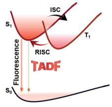
Fig. 1 Schematic diagram of the TADF mechanism.
