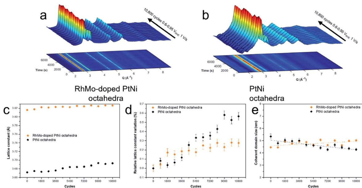
Fig. 4 3D representation and corresponding 2D projection of WAXS pattern intensities plotted as a function of time and the momentum transfer  $Q$  recorded in the AST (10,800 cycles between 0.6 and 0.95  $V_{\text{RHE}}$  at a scan rate  $1 \text{ V s}^{-1}$ ) for (a) oh-PtNi(RhMo) octahedra and (b) PtNi octahedra. Results from Rietveld refinement analysis in terms of the evolution of (c) the lattice constant, (d) relative lattice constant variation and (e) coherent domain size.
