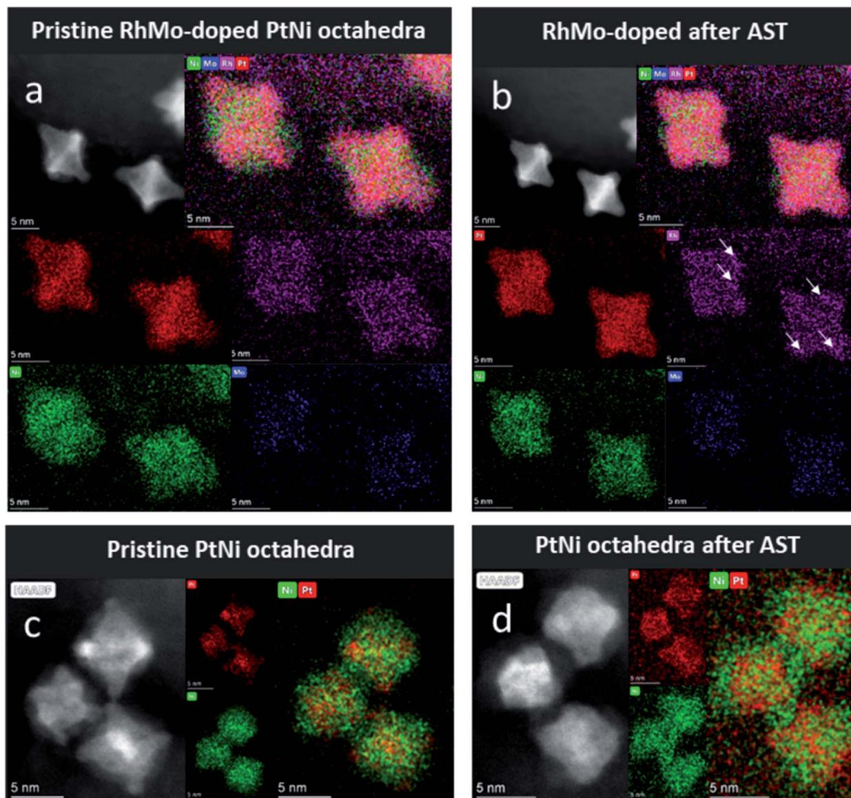
Fig. 3 IL-HAADF-STEM images (grey) and STEM-EDX composition maps of the pristine state (a) and (c) and after an AST of 10 800 cycles between 0.6 and 0.95  $V_{RHE}$  at a scan rate  $1 \text{ V s}^{-1}$  (b) and (d) for RhMo-doped PtNi (Pt in red, Ni in green, Rh in purple, and Mo in blue) and PtNi octahedra.
