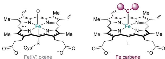
Fig. 17 Comparison of Fe-oxene and Fe-carbene intermediates in heme-based metalloenzymes proposed by Arnold.<sup>104,105</sup>
