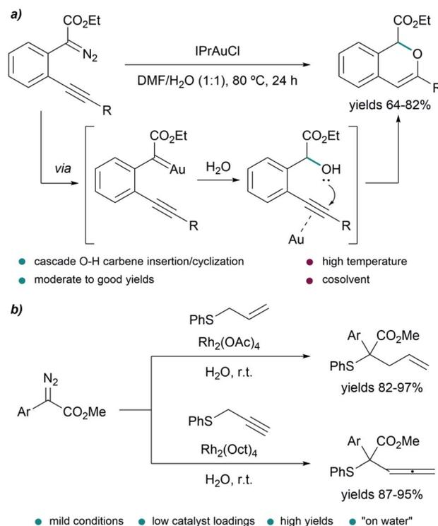
Fig. 6 (a) Gold-catalyzed tandem O–H insertion/cyclization in DMF/H<sub>2</sub>O. (b) Doyle–Kirmse reaction of *in situ* generated sulfonium ylides.
