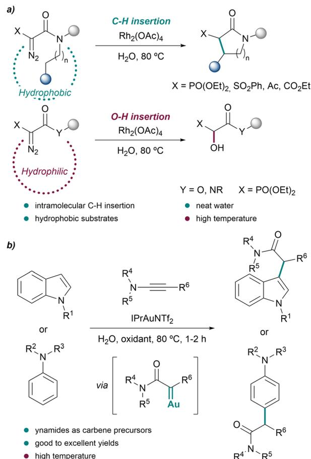
**Fig. 4** C–H insertion reactions in water. (a) Intramolecular insertion of rhodium carbenoids into aliphatic C–H bonds reported by Afonso and coworkers. (b) Functionalization of indoles and anilines by *in situ* generated  $\alpha$ -oxo gold carbenes.
