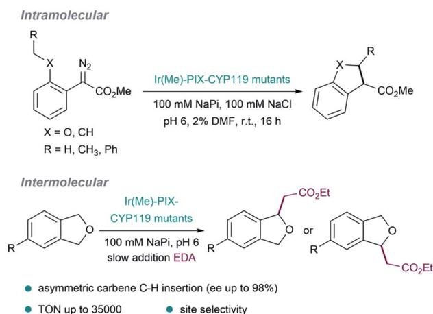
Fig. 10 Insertion of carbenes into C(sp<sup>3</sup>)–H bonds catalyzed by several metal–PIX reconstituted myoglobins containing a single mutation at the axial residue.
