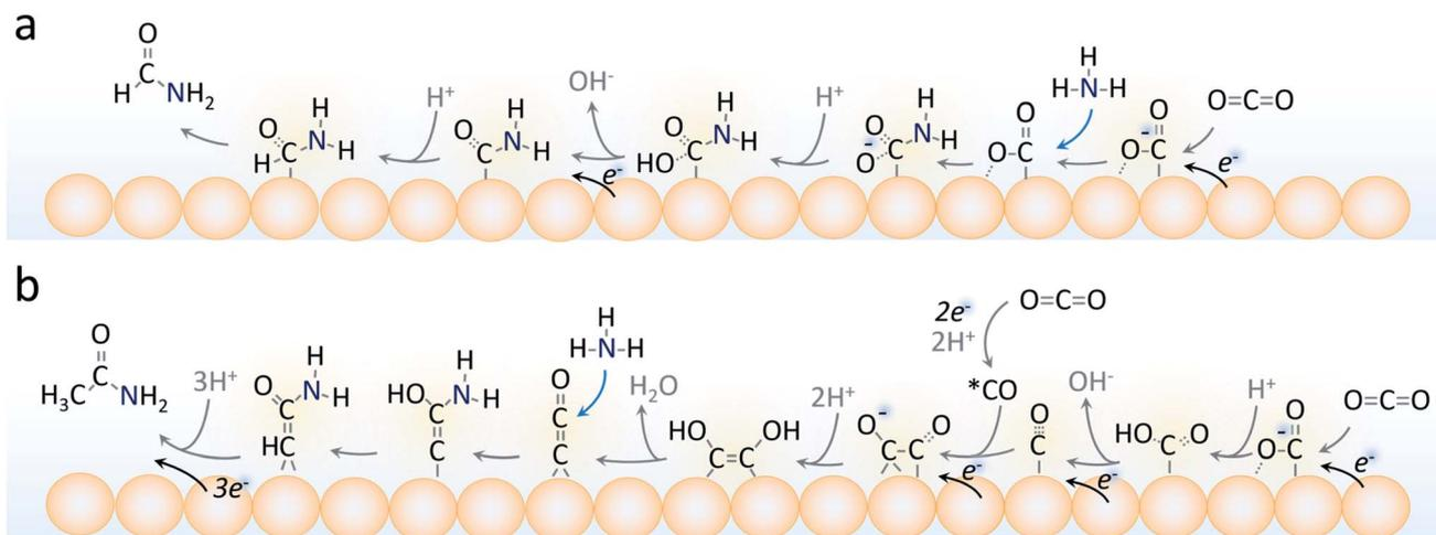
Fig. 7 Plausible surface reaction pathways in the electrochemical process of formamide (a) and acetamide (b) generation. Formamide generation depends on NH<sub>3</sub> coupling with the first reaction intermediate while acetamide generation requires highly reduced C<sub>2</sub> intermediates to be present on the catalyst surface. For simplicity, the donation of a proton to surface intermediates via H<sub>2</sub>O → OH<sup>-</sup> is depicted as →H<sup>+</sup>.
