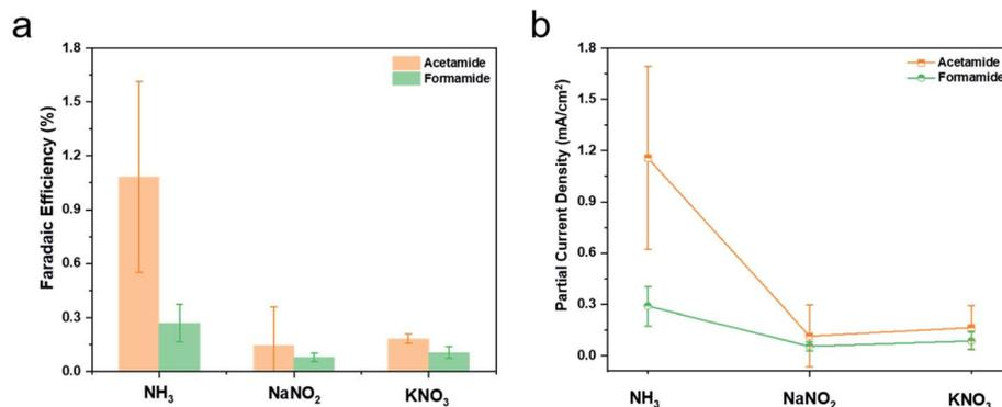
Fig. 5 In the equivalent reaction setup as in Fig. 3 with Cu catalysts and NO<sub>2</sub><sup>-</sup> (0.5 M) or NO<sub>3</sub><sup>-</sup> (1 M) in place of NH<sub>3</sub> at -0.98 V vs. RHE, formamide and acetamide were generated. The faradaic efficiencies (a) and partial current densities (b) for their generation were compared to those from using NH<sub>3</sub>.
