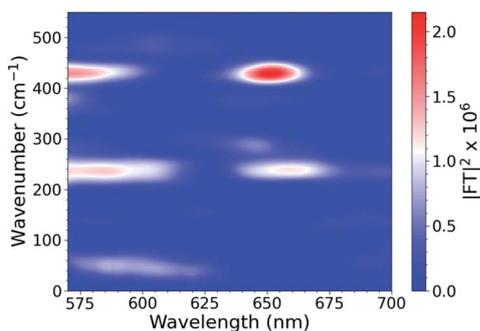
Fig. 3 ISRS spectra of CuOs following 540 nm excitation.
