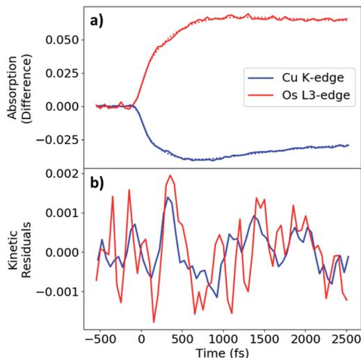
Fig. 5 (a) Kinetics traces for CuOs measured at Cu K (8.986 keV, blue) and Os  $L_{III}$  (10.871 keV, red) edges. Experimental data and fits shown as solid and dotted lines, respectively. (b) Filtered kinetic residuals, with Os residual inverted for comparison.
