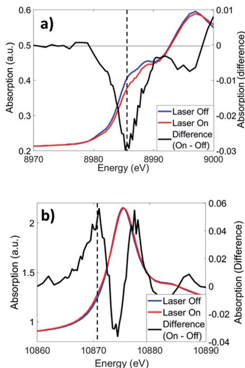
Fig. 4 XTA spectra of CuOs at the (a) Cu K-edge and (b) Os L<sub>III</sub>-edge at 2 ps and 0.7 ps time delays, respectively, following 500 nm excitation. Dotted lines indicate the energies used for kinetics traces in Fig. 5.
