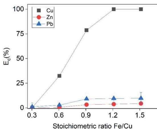
Fig. 5 Cementation efficiency of Cu as a function of the stoichiometric ratio Fe/Cu. Conditions:  $t = 30 \text{ min}$ ,  $[\text{Cu}]_i = 500 \text{ mmol L}^{-1}$ ,  $[\text{Zn}]_i = 23 \text{ mmol L}^{-1}$ ,  $[\text{Pb}]_i = 23 \text{ mmol L}^{-1}$ .
