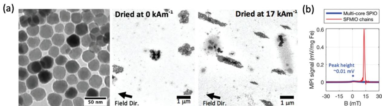
**Fig. 7** Microscale linear chain structures, designed for optimal MPI spatial resolution and sensitivity. (a) TEM images showing clear formation of microscale chain structures following application of an external magnetic field. (b) PSF demonstrating order-of-magnitude taller and sharper signal peaks for the chains over standard multi-core ferucarbotran, where SFMIO is a superferromagnetic iron oxide chain. Reproduced from ref. 14 with permission from Wiley-VCH.
