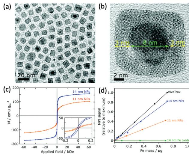
**Fig. 9** Stable Fe(0) nanoparticles, designed for optimal MPI performance. (a) Low and (b) high resolution TEM (HRTEM) images of the cubic 14 nm nanoparticles. (c) Hysteresis curves displaying the field-dependent magnetism of 14 and 11 nm Fe(0) nanoparticles. (d) Plot of the MPI signal of the synthesised samples in comparison to that of the reference, VivoTrax, as a function of core mass. Reproduced from ref. 1 with permission from the Royal Society of Chemistry.
