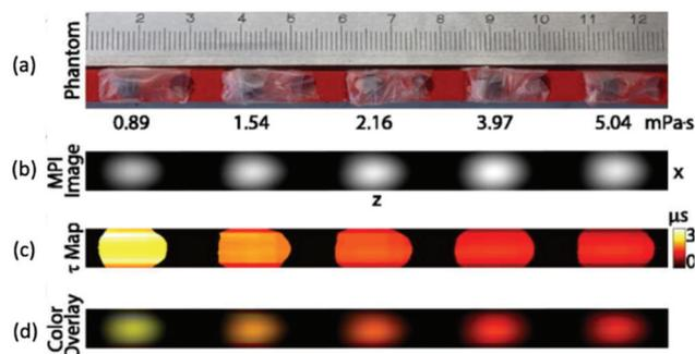
**Fig. 27** Multi-colour MPI images for viscosity mapping. (a) An imaging phantom of 5 different samples of SPIONs in increasing viscosity levels from 0.89 mPa s to 5.04 mPa s. (b) The MPI images for each sample, with (c) their corresponding relaxation ( $\tau$ ) maps. (d) The color overlay between the  $\tau$  maps and MPI images for each sample. Reproduced with permission of IOP Publishing, from ref. 22; permission conveyed through Copyright Clearance Center, Inc.
