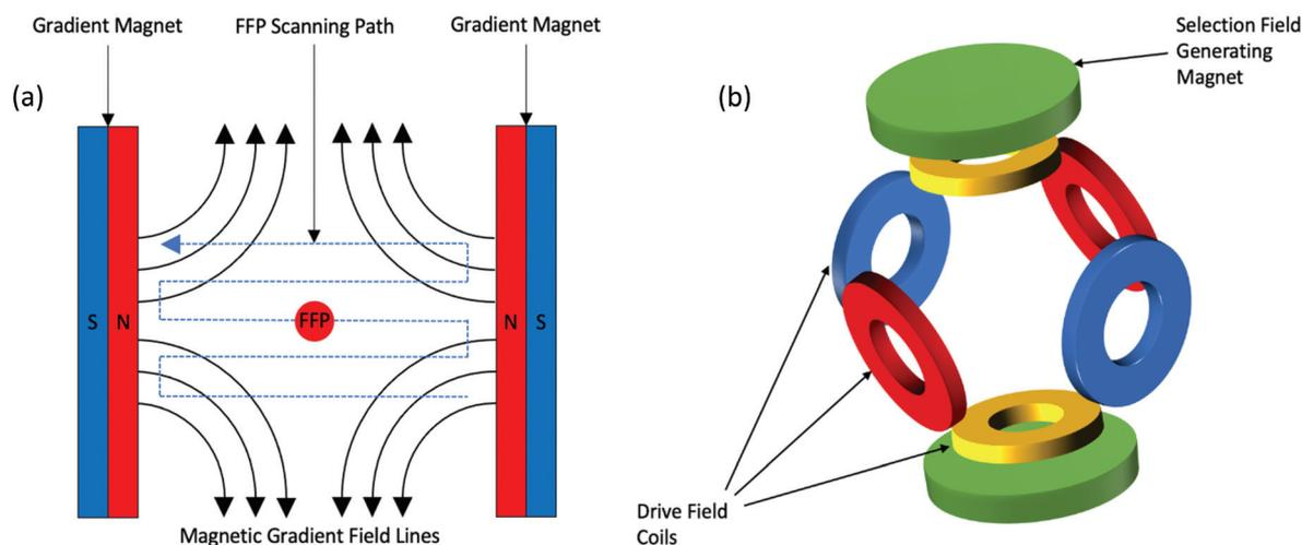
**Fig. 1** (a) The magnetic gradient field generated by an MPI scanner with two permanent magnets, producing an FFP along with magnetically saturating regions. The FFP is rapidly scanned over the FOV *via* variation of the drive field, generating signal from the reorientation of the SPIONs magnetisation. (b) Configuration of drive field coils required to generate a drive field.
