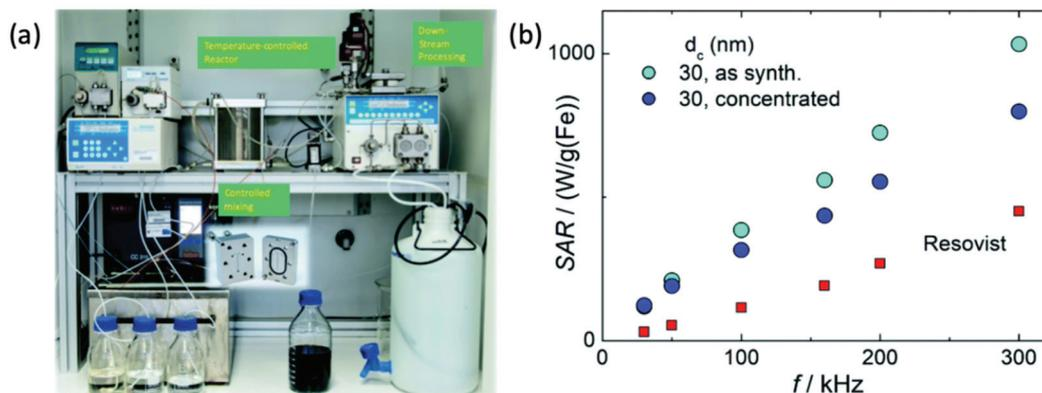
**Fig. 22** MPI-tailored single-core SPIONs, designed for MPI–MFH. (a) Photograph of the micromixer system used for the synthesis of 30 nm monodisperse single-core SPIONs. (b) SAR values of the synthesised SPIONs as a function of frequency ( $f$ ), in comparison to that of the reference, Resovist. Reproduced with permission of the Royal Society of Chemistry, from ref. 9; permission conveyed through Copyright Clearance Center, Inc.
