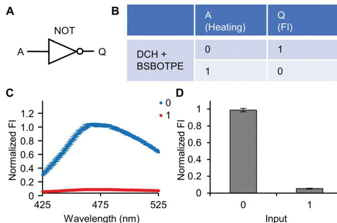
**Fig. 5** NOT logic operation. (A) Symbol of logic gate. (B) Truth table. (C) The normalized fluorescence spectra of logic operation with different inputs. (D) Normalized FI at 471 nm. The concentrations of DCH and BSBOTPE used are 6  $\mu\text{M}$  and 141  $\mu\text{M}$ , respectively. Excitation wavelength was set at 350 nm. The 'heat' input is incubated under 40  $^{\circ}\text{C}$  for 2 min.  $n = 3$ .
