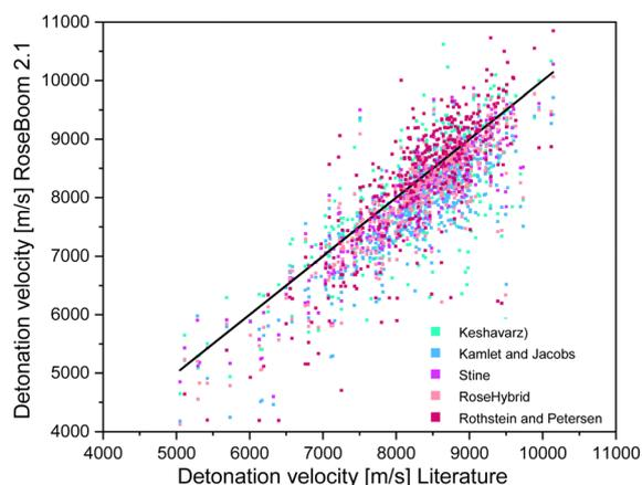
Fig. 6 Scattering plot of the detonation velocities predicted with the methods implemented in RoseBoom2.1<sup>©</sup>, plotted against the literature values.
