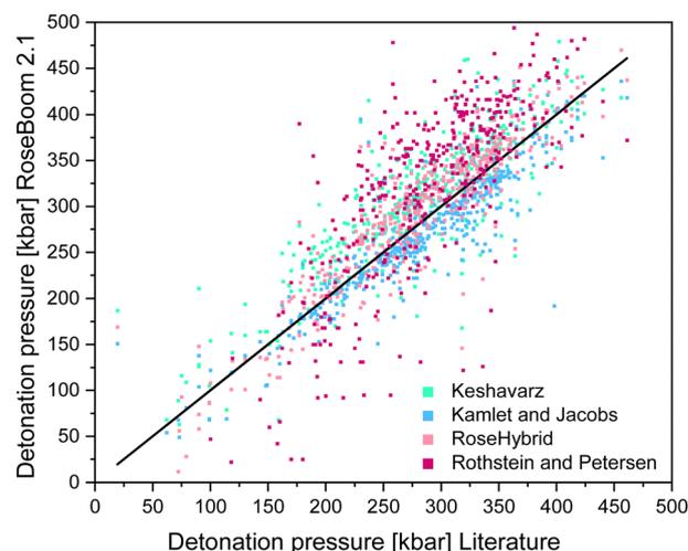
**Fig. 7** Scattering plot of the detonation pressures predicted with the methods implemented in RoseBoom2.1<sup>©</sup>, plotted against the literature values.
