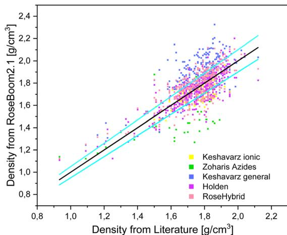
Fig. 8 Scattering plot of the densities predicted with the methods implemented in RoseBoom2.1<sup>©</sup>, plotted against the literature values and sky-blue errorbars of 5%.
