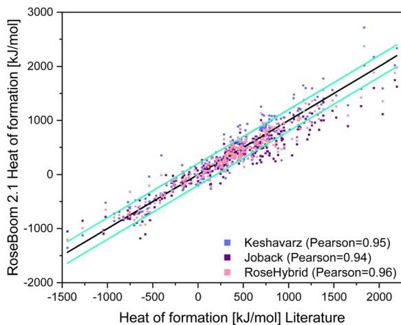
**Fig. 10** Scattering plot of the heat of formations predicted with the methods implemented in RoseBoom2.1©, plotted against the literature values, with turquoise error bars marking a range of  $\pm 200$  kJ mol<sup>-1</sup>.
