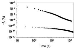
Fig. 7 Retention time of the  $I_{\rm d}$  of the OFET memory device with TIPS-pentacene/CuSP blend films, as monitored at  $V_{\rm g} = -5$  V after writing (black squares) and erasing (white circles) operations.
