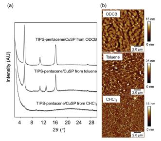
Fig. 2 (a) XRD profiles of TIPS-pentacene/CuSP blend films spin-coated from various solvents. (b) AFM height images of the TIPS-pentacene/CuSP blend films
