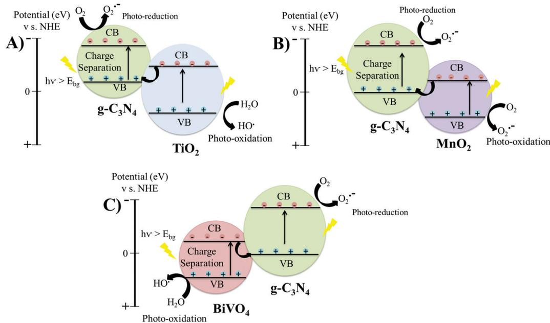
Fig. 6 Schematic of band structures and charge transfer mechanism in direct Z-scheme heterojunction structures: (A)  $g\text{-C}_3\text{N}_4\text{-TiO}_2$ ; (B)  $g\text{-C}_3\text{N}_4/\text{MnO}_2$ ; and (C)  $\text{BiVO}_4/g\text{-C}_3\text{N}_4$ .
