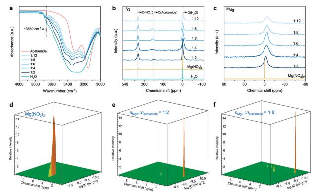
Fig. 2 Spectroscopic characterizations of the electrolytes. (a) FT-IR, (b) liquid-state <sup>17</sup>O NMR, and (c) liquid-state <sup>25</sup>Mg NMR spectra. PFT-NMR contour spectra of (d) 1 M Mg(NO<sub>3</sub>)<sub>2</sub>, (e) the electrolyte with  $n_{\text{Mq}^2+}$ :  $n_{\text{acetamide}} = 1:2$ , and (f) the electrolyte with  $n_{\text{Mq}^2+}$ :  $n_{\text{acetamide}} = 1:8$ .
