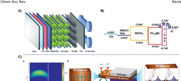
Fig. 8 (A) Device configuration of CON/PEDOT: PSS HTL incorporated PSC. Reproduced with permission from ref. 87. Copyright 2018, Royal Society of Chemistry. (B) Device incorporating T-POP as a secondary ETL. Reproduced with permission from ref. 90. Copyright 2020, Elsevier. (C) GIWAXS plot with device configuration. Reproduced with permission from ref. 92. Copyright 2021, American Chemical Society.
