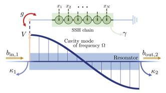
Fig. 1 Schematic picture of a dimerized chain interacting with the photons in a cavity, of frequency  $\Omega$ . The cavity is connected to the input and output ports l = 1, 2 with factors  $\kappa_i$  (i = 1, 2). Fermions and photons interact with coupling strength q, while  $\gamma$  represents the spectral broadening of the fermionic system.
