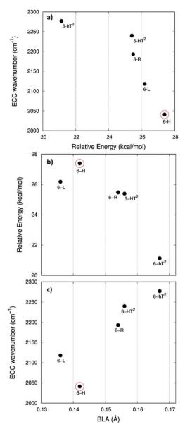
Fig. 5 Correlation between physical quantities sensitive to  $\pi$ -electrons conjugation. Panel a: ECC phonon wavenumber vs.  $\Delta E$  ( $\Delta E$  is the relative crystal energy – per atom – referred to graphene, see text). Panel b:  $\Delta E$  vs. BLA parameter. Panel c: ECC phonon wavenumber vs. BLA. The data corresponding to 6-H crystal is highlighted by a red circle.
