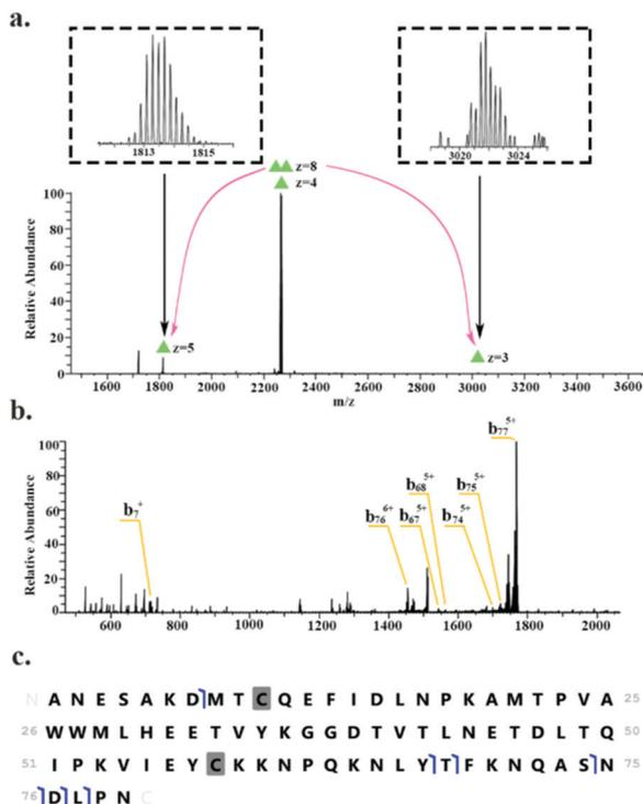
Fig. 3 Identification of the HdeB homodimer. (a) HCD MS/MS (35% NCE) of 8+ precursor ions ( $m/z$  2266.6  $\pm$  4) results in dissociation of dimer to monomer (5+ and 3+ charge states). (b) HCD MS/MS of 5+ monomer ions ( $m/z$  1813.5). (c) Summary of sequence fragments observed.
