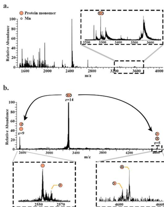
Fig. 4 Native LESA mass spectrum of Mn-bound superoxide dismutase dimer. (a) Full scan mass spectrum with enlarged  $m/z$  region showing the peak corresponding to superoxide dismutase dimer. (b) HCD of the 14+ precursor ions ( $m/z$  3289.5  $\pm$  6) results in dissociation of the dimer to monomer (9+ and 5+ charge state) with differing numbers of  $Mn^{2+}$  bound.
