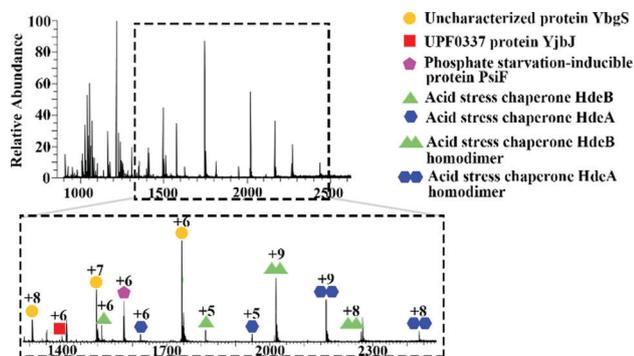
Fig. 1 Representative mass spectrum acquired by native LESA MS following electroporation of *E. coli* K12 colony.
