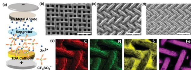
Fig. 3 (a) Schematic model of Zn-HSC energy storage system. (b) SEM image of pure stainless steel electrode. (c) SEM image of **TDA-1** on stainless steel electrode. (d) SEM image of **TDA-2** on stainless steel electrode. (e) Element mapping spectra of C, N, S, Fe on **TDA-1** electrode. Scale bars of (b–d) correspond to 200  $\mu\text{m}$ .
