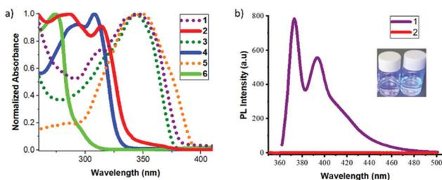
**Fig. 1** (a) UV-Vis spectra of **1–6** in THF ( $3 \times 10^{-5}$  M to  $1 \cdot 10^{-6}$  M). (b) Fluorescence emission spectra of **1** and **2** in THF ( $3 \times 10^{-5}$  M to  $1 \times 10^{-6}$  M). Inset: Solutions of **1** and **2** in THF under UV irradiation.
