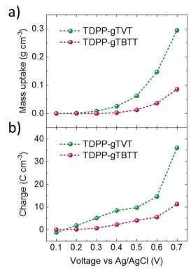
Fig. 3 Electrochemical guartz crystal microbalance with dissipation monitoring (EQCM-D) results of TDPP-gTVT and TDPP-gTBTT. The differences in (a) the electrolyte uptake and (b) charge generation per unit volume during the application of doping potentials from 0.1 V to 0.7 V vs. Ag/AgCl with a step of 0.1 V.
