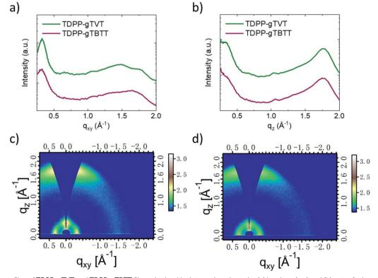
Fig. 5 Line-cut profiles of **TDPP-gTVT** and **TDPP-gTBTT** films obtained by integration along the (a) in-plane  $(q_{xy})$  and (b) out-of-plane  $(q_z)$  direction. 2D grazing-incidence wide-angle X-ray scattering (GIWAXS) images of (c) **TDPP-gTVT** and (d) **TDPP-gTBTT** films;  $q_z$  and  $q_{xy}$  are the perpendicular and parallel wave vector transfers with respect to the substrate surface.
